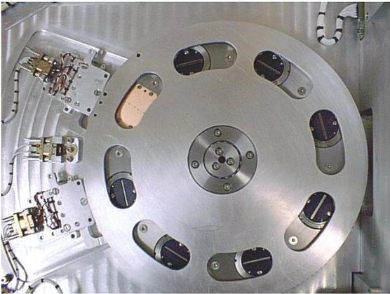
Fig 2: Slit rotation/selection mechanism
