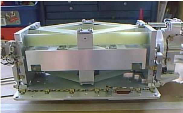
Fig 6: Detector focus/translation mechanism
