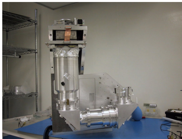
Figure 3. GPI spectrograph before cryogenic testing.
